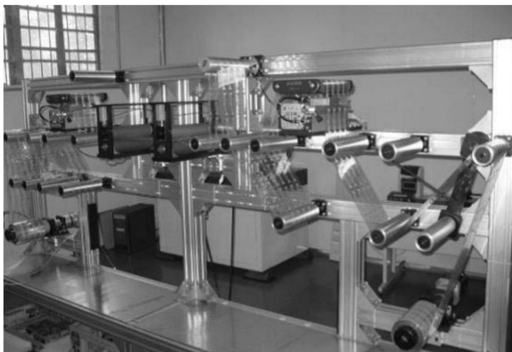
Figure 12. Image of a Roll-to-Roll (R2R) setup in a clean room environment with different printing process units installed in the production line [11]
