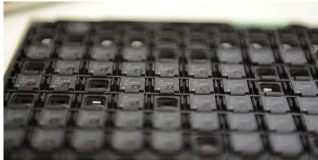
Figure 7. Network of PULP microprocessor chips on a tray. PULPino chips are smaller, depending on technology and memory size as small as 1 x 1 millimeter. Credit: ETH Zurich [5]
